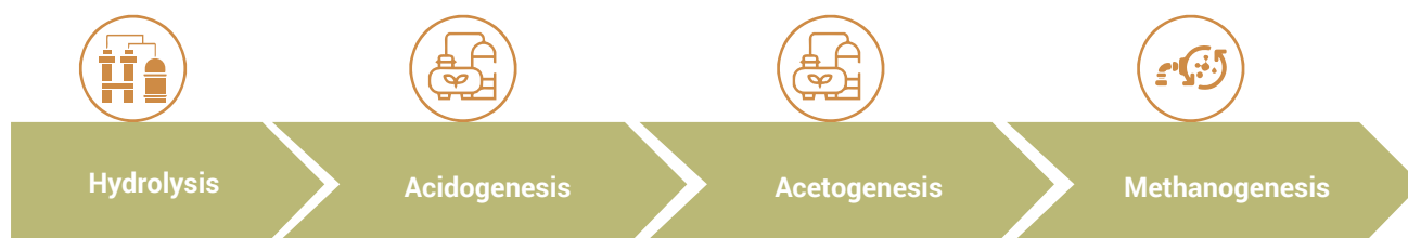
Figure 6: Bio-chemical process flow for biogas production
