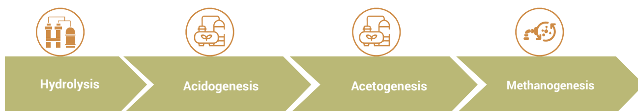
Figure 6: Bio-chemical process flow for biogas production
