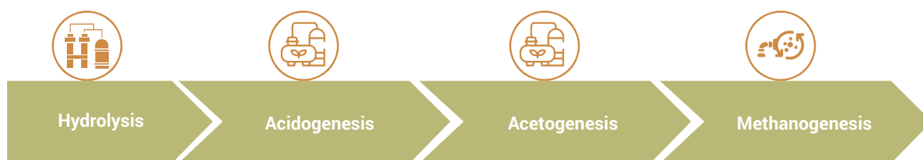
Figure 6: Bio-chemical process flow for biogas production
